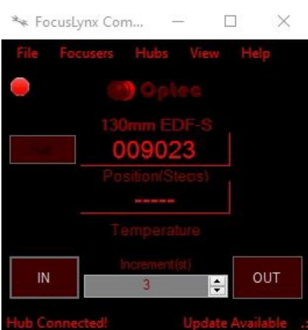
This software also connects to parts of the telescope and keeps a given object in focus. Using FocusLynx there is no need of keeping the object focused manually. This is valuable as often as in our case, the object is too dim to see properly without enough illumination time with a camera.
