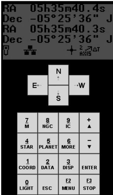
This software allows us to control the telescope with a PC. It is a mirror of the attached keypad, which allows remote control from inside a house, without giving up monitoring of the telescope. It shows status, and the direction in which the telescope is pointing.
