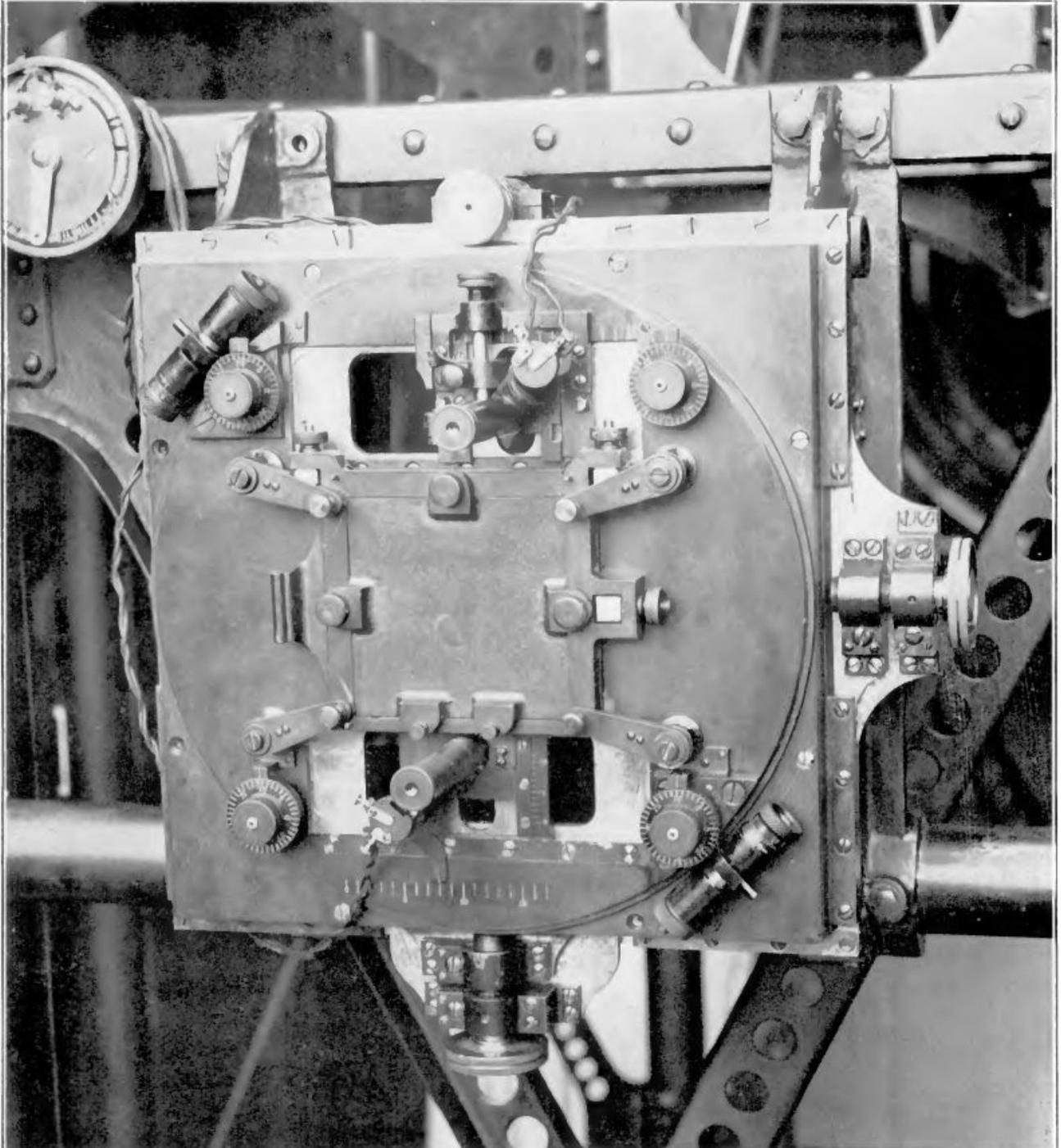
*Fig. 23: photographic plate-carrier*
